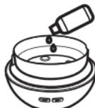
2. Remove the cover, add water. Then add 2-3 drops of essential oil. Note that if the water level exceeds the maximum limit, mist may not come out.
